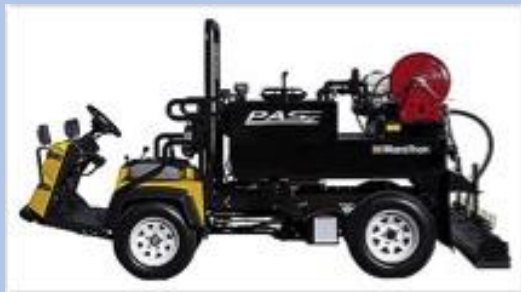
Bitumen spreading machine
